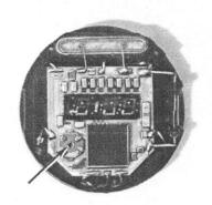
Front of module. Note flat rough-adjustment trimmer.
