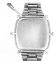
**3.** When screws are removed, carefully remove case back and gasket. Note cell arrangement — two (at top) are free, two (in center) are held by L-shaped clamp.
