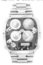
Be sure cells are located properly in accordance with the "+ UP" and "+ DN" markings in each cavity, as pictured above. Re-position L-clamp as shown and tighten screw.
