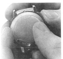
**6.** Replace case back, making sure the small tab is properly seated in the slot at the "12 o'clock" position. Press back into place and hold with fingers of left hand.
