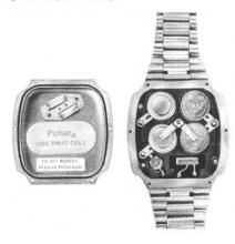
**4.** Examine cell connector in case back to make sure it is fastened securely.
