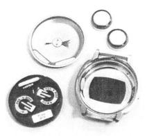
Remove module from case before ultrasonic cleaner.
