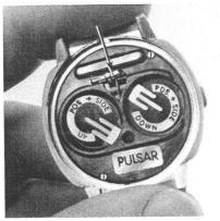
Back of module. Note fine-adjustment trimmer.
