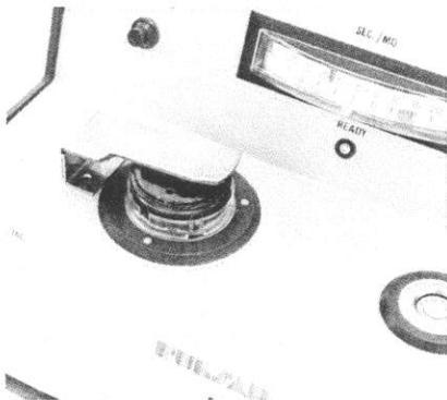
7. Place service case with module on Pulsar Analyzer, **power cells down**, and position it so you have access with rough-trimmer tool to hole over rough trimmer.
