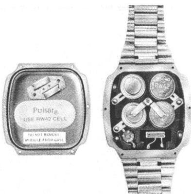
4. Examine cell connector in case back to make sure it is fastened securely.
