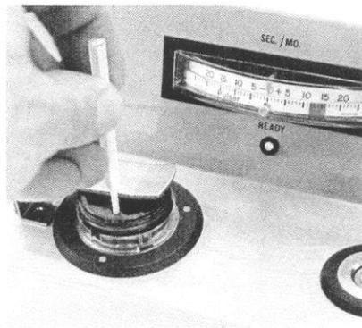
8. Insert rough trimmer tool into center of rough-adjustment trimmer. Turn until the Pulsar Analyzer meter indicates plus or minus 2 seconds/month.
