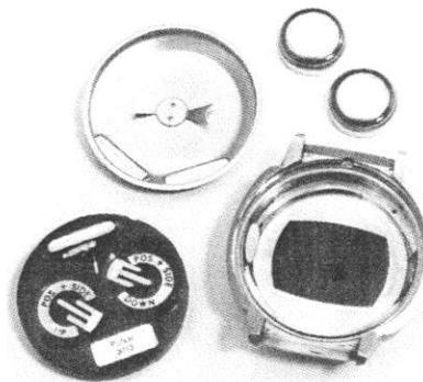
Remove module from case before ultrasonic cleaner.
