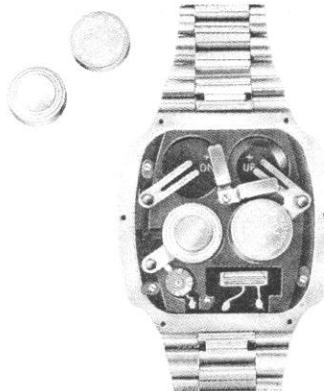
Do not loosen clamp fully or remove it from module. If clamp is removed accidentally, be sure to replace it properly — with the long lead **under** the double connector in the lower left cell cavity.
