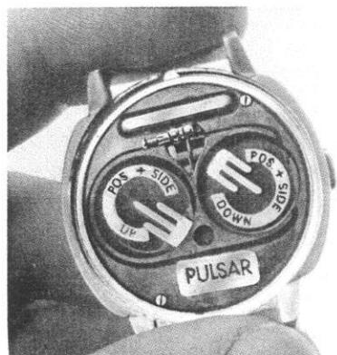
**4.** Remove old power cells, and replace with new cells. Cell holders are marked "plus side up" and "plus side down," referring to the "plus" sign on one side of each power cell. Be sure cells are placed accordingly.
